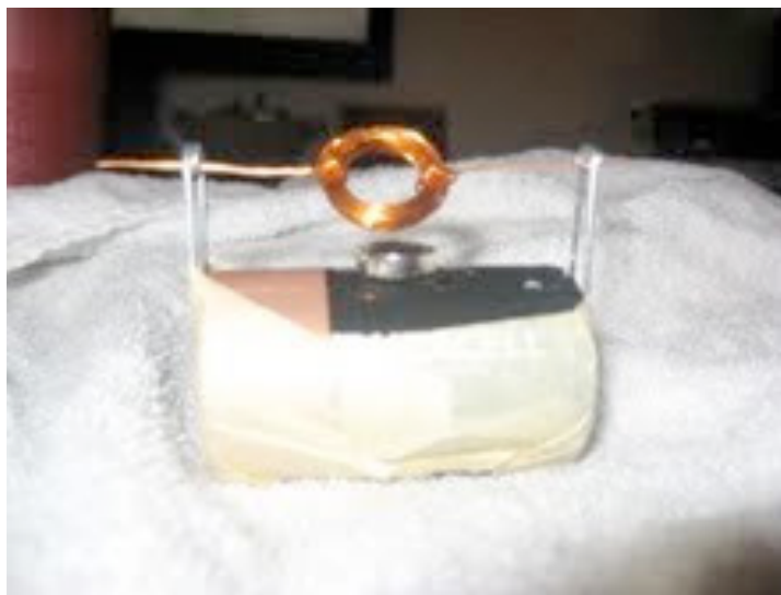
Figure 1 - the finished electromotor
